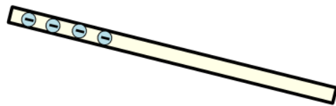
This polythene strip has a negative electric charge.
